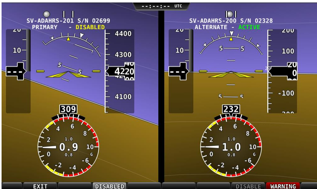
Figure 56 - ADAHRS Cross-Check Comparison (one ADAHRS disabled)
