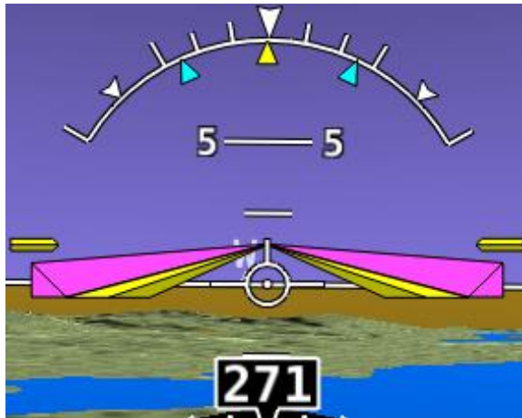
Figure 206 - Single Cue / Inverted-V with Autopilot Servos Engaged
