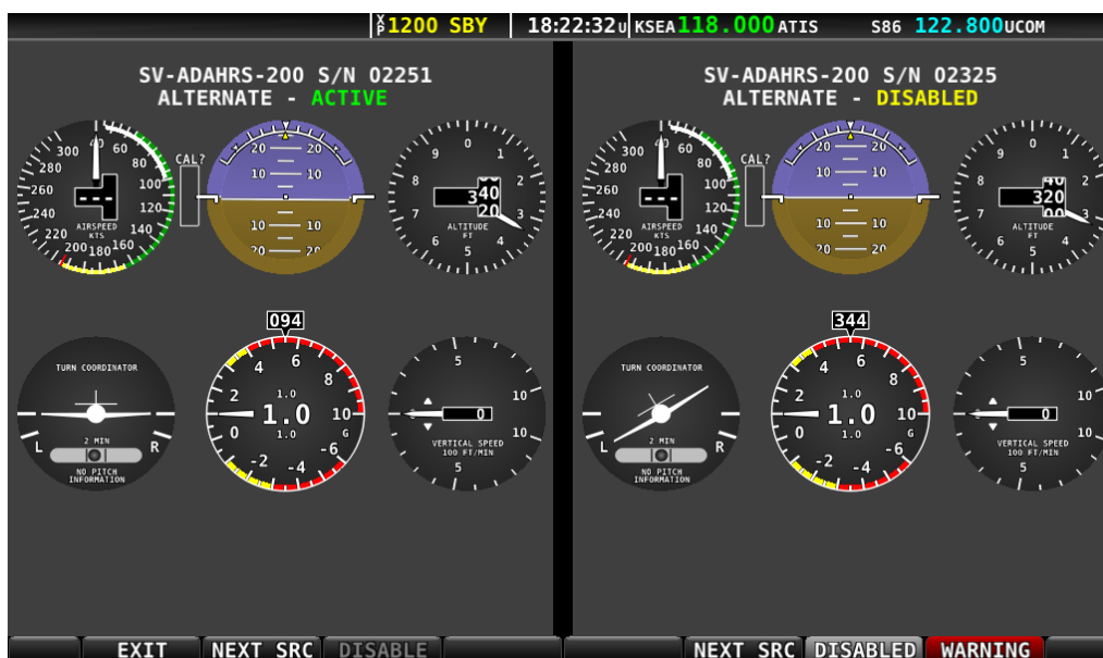
Figure 57 - ADAHRS Cross-Check Comparison – six-pack
