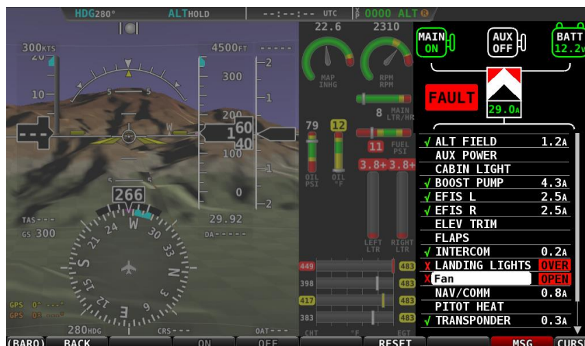
Figure 73 - VP-X Page with Fault
