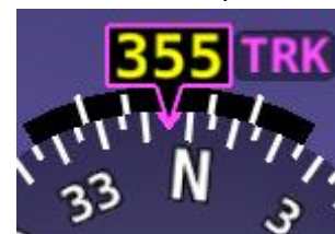
Figure 23 - GPS Track substitute for Magnetic Heading
