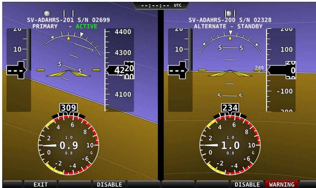
Figure 55 - ADAHRS Cross-Check Comparison
