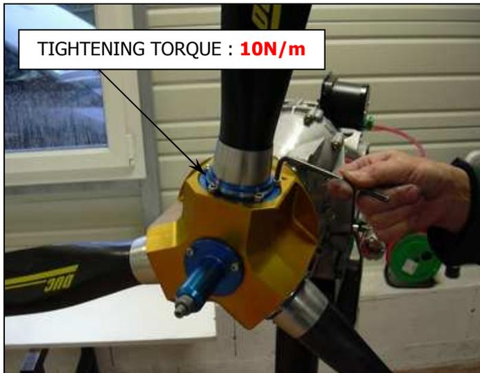
Block the 5 brake screw CHC M6 to the tightening torque of 10 N/m.
